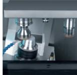
Two tool spindles enable rough and fine grinding in one process cycle including centering and beveling.
