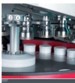
The CNC controlled tool changer allows multiple step processing.
